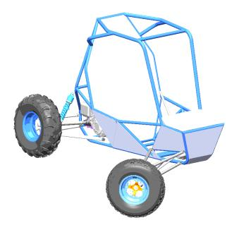
Current design of the 16x, featuring a newer, lighter frame and significant rear suspension improvements! (Don't worry, the real thing will have 4 wheels.)
